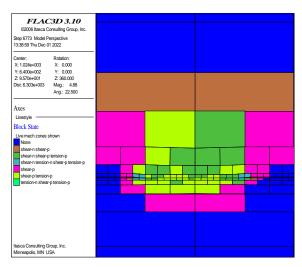
Figure 4: Damage zone distribution around the gob.
