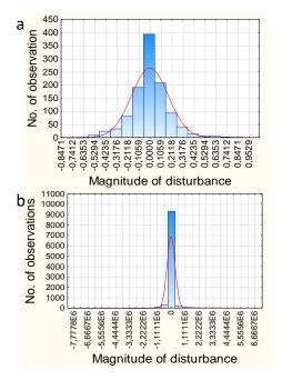
Figure 3: Distribution of the disturbance: a) simple model; b) complex model: STD is 10% and 3% correspondingly.
